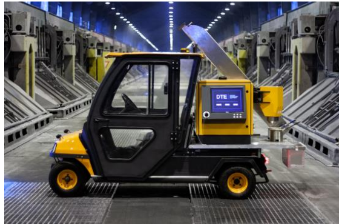
Figure 1. DTE's portable elemental analyzer.
